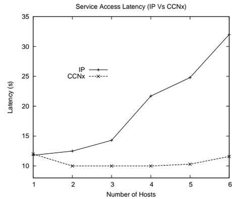
Fig. 10. IP vs CCNx service access latency.
