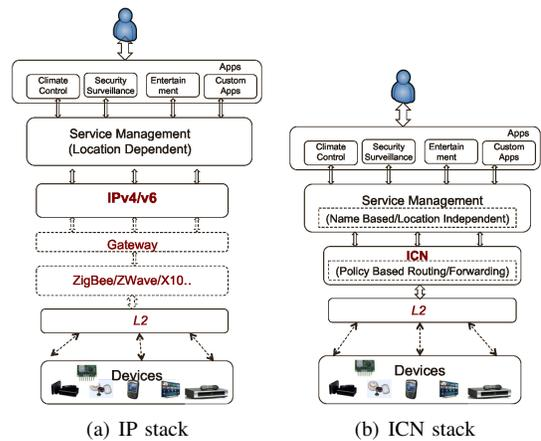
Fig. 2. IP vs ICN homenet stack.
